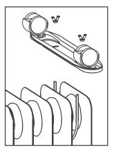
Operate heater in upright position only (wheels on bottom, controls on top). Any other position could create a hazardous situation.
