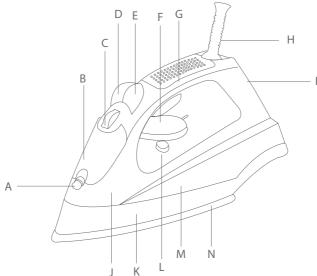
A. Spray Nozzle B.Water filling inlet C.Steam control dial D. Burst of steam button E.Spray Button F. Temperature control dial G.Up cover H. Power cord protector
