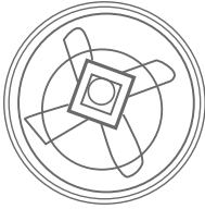
Wrong assemble of blade
