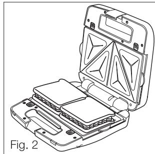
**Note:** Do not overfill with food-forcing the lid closed can break the clip.
